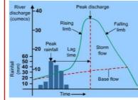
Rising limb = indicates discharge increases a few hours after rainfall. Peak flow = Discharge reaches max levels.
